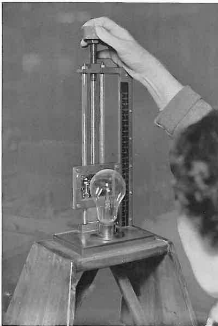
Measuring the light-centre length ensures that the filament is in exactly the correct position. With pearl lamps the filament position is checked by projecting a shadow of the filament on to the wall of the bulb.
