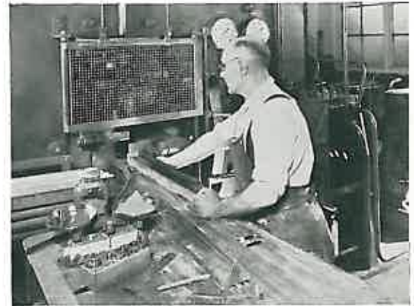
Powdered tungsten is converted into metal bars by compression in this press and by pre-sintering in a furnace.
