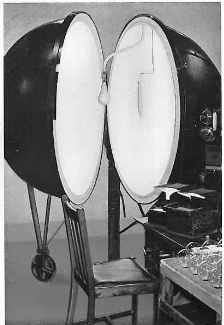
An integrating photometer—a perfect sphere used in conjunction with a photo-electric cell—is used to measure the total amount of light emitted by the lamp.
