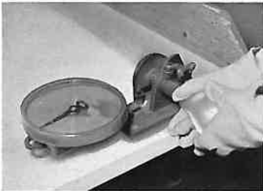
The glass neck of a Mazda lamp has moulded ridges which provide a key for the special heat and damp resisting cement which holds the cap. The firmness of cap fixing is put through this torsion test.
